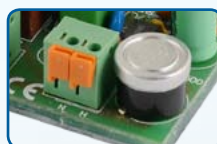
Termostat biometaliczny T_{ON}=15^{\circ}\text{C} , T_{OFF}=25^{\circ}\text{C}
